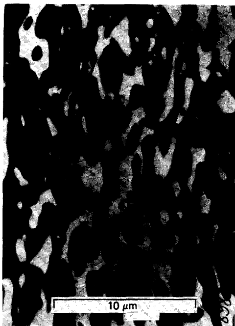
Figure 10 Transitional morphology of a 60 vol% EPDM (AP 447) containing PP blend (TEM)
